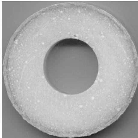
**Cut through propellant segment**
