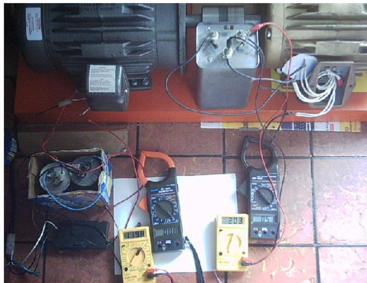
To measure the current relation in a RV, use 3 current shunts (can be resistors) 0.1 ohm in WYE. One leg goes to the source battery, one to return (generator to be tested, DC output), and the third to the load (inverter). A common ground is used for all devices (G).
