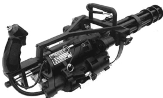
The M88 mini gun is a 10mm full automatic platoon support weapon. It has a cyclic rate of about 1800rpm. The M88 has two fire setting: safe or full automatic. Ammunition is stored on a roll of continuous plastic non-disintegrating link belt in the ammunition drum.
